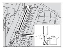
5 Return the transfer charger cleaner into the cleaner pocket, and then close the transfer unit.
